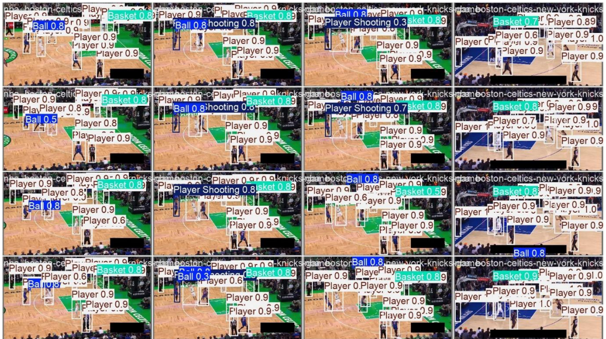
Figure 13 Sample validation predictions showing all five classes detected
